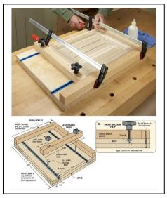
Finally the adjustable fence is added. It's held in place with flange bolts and star knobs. A couple of coats of paste wax completes the jig and keeps glue from sticking to the base and fences.
