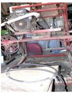
The photos show it clearly. There was a nail laying horizontally in the centre of the log and the blade had hit it end on and cut through the length of it, lost all sharpness and dived, pulled off the wheel and done its damage to the belt.
