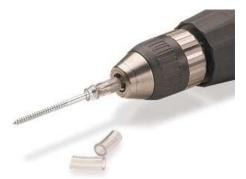
better solution I came up with the sure-fire screw gripper you see in the photo above It's simply a short length of soft plastic tubing. As you can see, the tubing slips snugly over the driver bit to hold the head of the screw firmly in place. Now, the screw can't get away, come out of the bit or go off line, and a sometimes frustrating job becomes easy.
